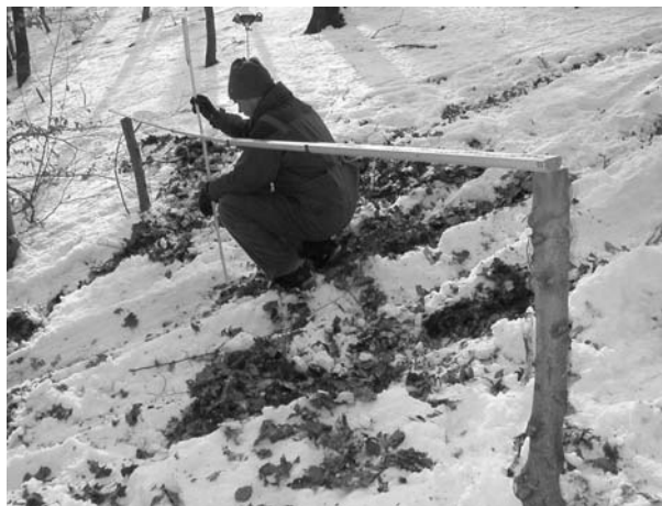
Figure 3. Measuring of rut depth.
