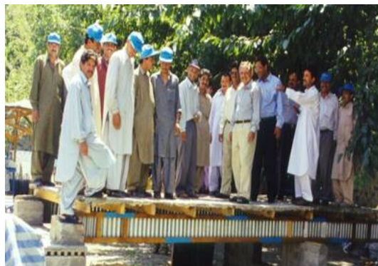
Picture 5: Demonstration of the Composite beam's load bearing strength
