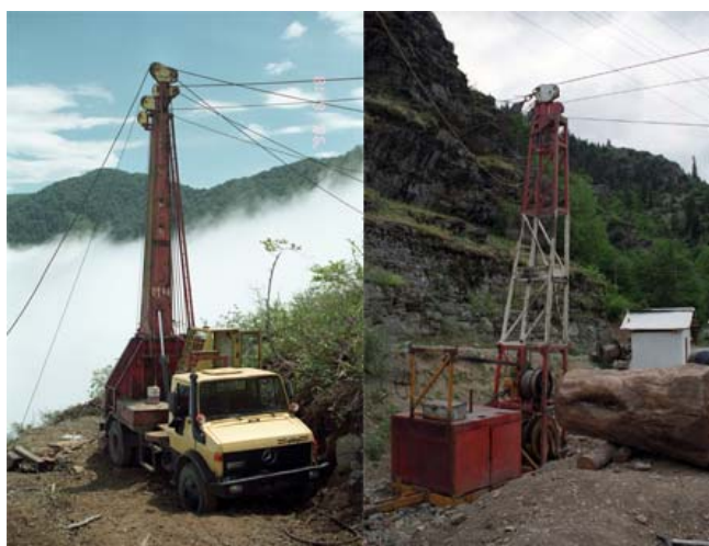
Figure 1. Typical tower yarders used in northeastern Turkey (left: URUS MIII, right: Koller K300).
